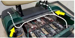
7. Route the front portion of the harness through the vertical channel on the driver side. Secure with cable ties.
