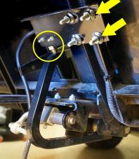
4. Slide the brake switch wire and the brake lead from the deluxe harness behind the bracket and down the channel with the existing harness.
