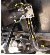
Install the LGT-142, time delay, near the first opening in the frame. Mark the hole location and drill an 1/8" pilot hole. Drill a 1/4" hole through the pilot hole. Mount the time delay with the <u>Included Hardware</u>.
