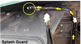
10. Remove the two rivets on the key switch plate and remove the plate to access the dash compartment.
